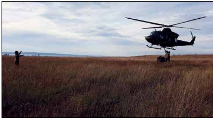
11th Field Regt Gunnery hook up ammo sling load, on Ex AUTUMN GUNNER.
