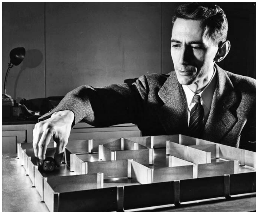
FIGURE 4. Claude Shannon demonstrated his maze-running “mouse,” Theseus, an early form of artificial intelligence, to the Macy conference on cybernetics in 1951. It showed that the logic elements used in the telephone system and in early computers (electromechanical relays) could simulate animal learning. Courtesy of AT&T Archives and History Center.
