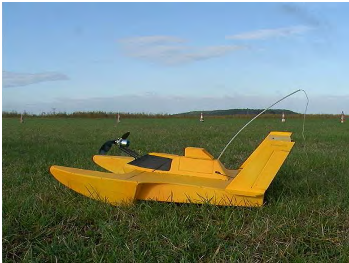
Le moteur brushless Flyware REX 220-1300 est placé à l'avant et l'hélice GWS 8x4.3 est en prise directe. The brushless motor Flyware REX 220/1300 is placed in front and the propeller GWS 8x4.3 is in direct drive.
