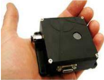
Fig 1: Integrated highly coherent VeCSEL with driving electronics
