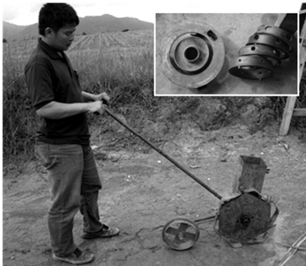
Figure II.4 Manual wheel NT planter (Brazil) suitable for the sowing in line of various crops under limited soil mulch conditions.
