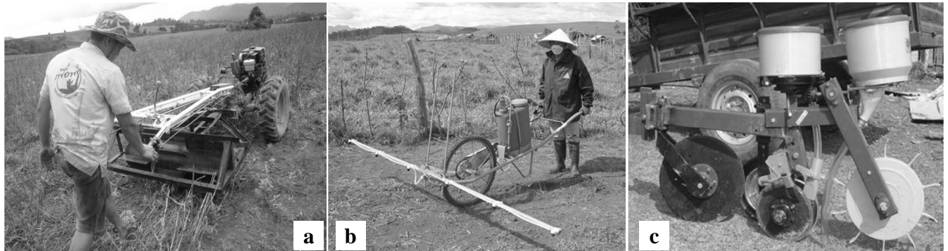
Figure II.1 CA implements used for land preparation and sowing: a) locally-made rolling knife for two-wheel tractor, b) 20L wheel sprayer (Knapick, Brazil), and c) 1-row NT planter (Fitarelli, Brazil) adapted for two-wheel tractor
