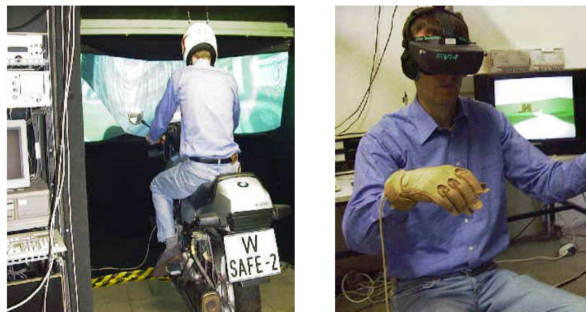
Fig. 7C.5: Motorcycle-simulator using VR-technology at the Chair of Safety of Transportation Systems
