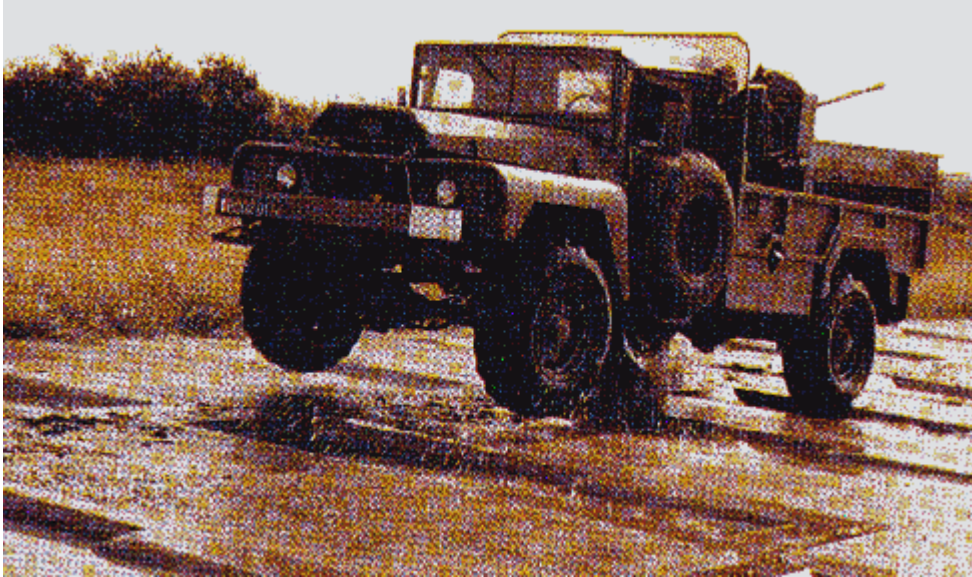
Figure 2: Example of special track (pothole) in Etablissement technique d'Angers (ETAS)
