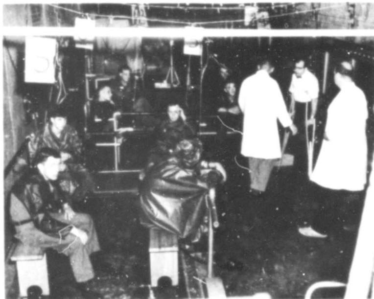
A. Volunteer subjects wearing a variety of raincoats, during a rest period inside the tropic environment test chamber
