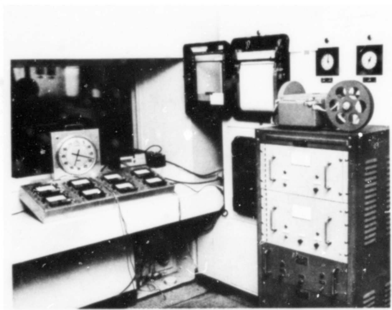
B. The physiologic data acquisition system for the environmental chamber
