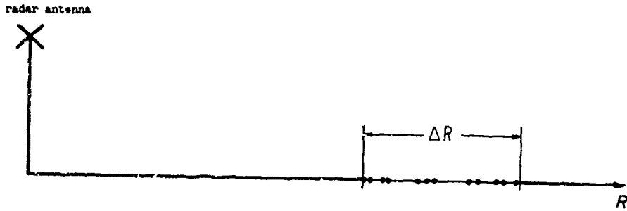
Fig. 11 Backscatter model with 12 statistically distributed "high-lights"
