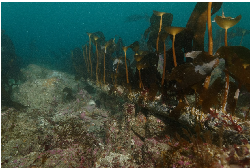
Figure 3: Colonisation of the cable deployed in a rocky environment of the SABELLA tidal test-site (France). A high density of kelps ( Laminaria hyperborea ) was observed on the naked cable (Credits: Olivier Dugornay – IFREMER).
