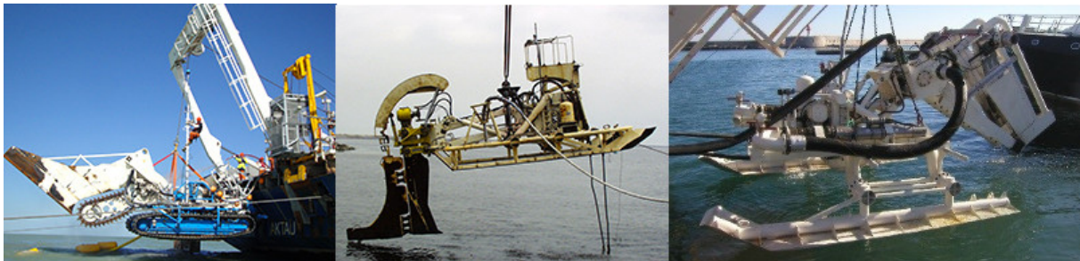
Figure 1: Wheel cutter (left); Plough (centre) and Towed Jetting Vehicle (right) (courtesy: www.ldtravocean.com ).
