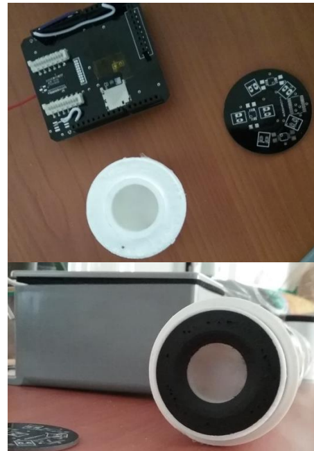
Fig. 3. Components and assembled optical sensor.
