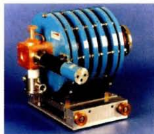
SUPERANOGAN: An ECR source with permanent magnet for low and high charge state. (H + : 2mA, A m+ : 350µAe)
