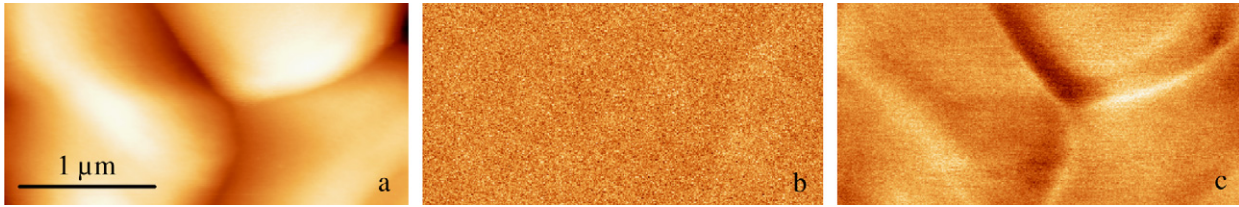
Fig. 3. Topography (a), CPD measured with a lift (b) CPD measured with a linear scan mode (c) of the same area of a sputtered Al layer. Peak to valley values are respectively 66 nm, around 8 meV (noise level) and 27 meV. To allow comparison, potential color scales are identical.
