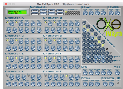
Figure 136 OXE 8-operator FM software synthesizer. Note the “modulation matrix” at right, whose lower-diagonal structure implies a full DAG is possible but not a cyclic graph except for self-modulating operators.
