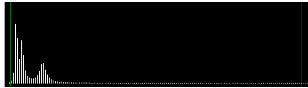
Figure 126 First three male voice formants for an “Ahh” sound, as simulated by three resonant bandpass filters added together. Note the differences in frequency, amplitude, and bandwidth among the three filters.
