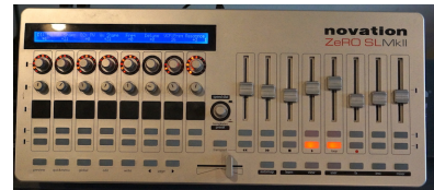
Figure 173 Novation Remote Zero SL Mk II, with assignable dials, buttons, sliders, and drum pads.
