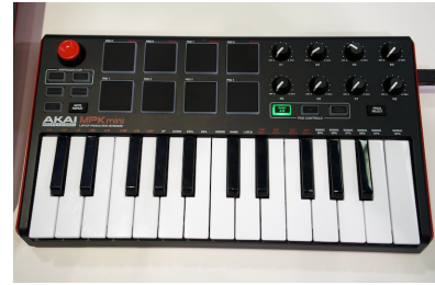
Figure 172 Akai MPK mini MIDI controller, with a self-centering joystick (red), drum pads, assignable knobs, and velocity sensitive mini keys. ©70
