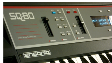
Figure 177 Ensoniq SQ80 synthesizer, one of the few synthesizer keyboards with polyphonic aftertouch. ©74
