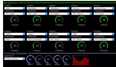
Figure 41 Screenshot of part of the Edisyn patch editor for the Oberheim Matrix 6, showing (at top) its 10-entry modulation matrix. Each entry has a source, a destination, and a modulation amount. At bottom is the Matrix 6 tracking generator, a form of modifier function. The Matrix 6 is discussed in more detail in Section 5.3.
