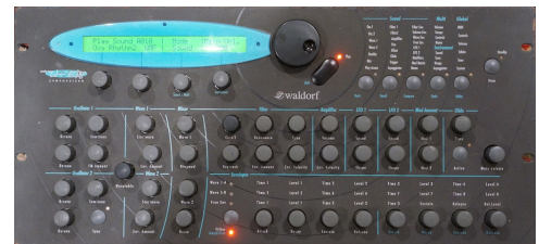
Figure 143 Waldorf Microwave XT (rare "Shadow" version: most were safety orange!). Note the bottom right quadrant of the knob array, devoted entirely to envelopes.
