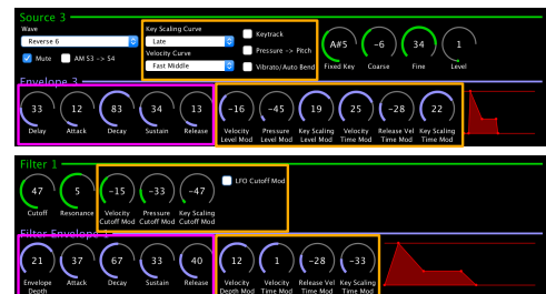
Figure 40 Screenshots of portions of the Edisyn patch editor of the Kawai K4 for (top) one oscillator and (bottom) one filter. Orange boxes indicate K4 parameters for hard-coded modulation routings. Purple boxes indicate parameters of dedicated envelopes for amplitude (top) and filter cutoff (bottom). The remaining regions were the actual oscillator and filter parameters.
