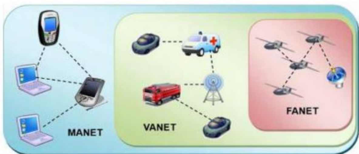
Figure 10 : Architecture de MANET, VANET et FANET (49)
