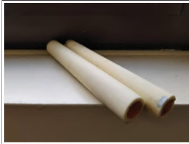
Figure 3.2 True Phantom Solutions human bone mimicking phantoms ; healthy bone phantom on the left, osteoporotic bone phantom on the right
