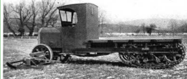
Side View of the Linn Self-Laying Track, Geared-to-the-Ground Tractor This tractor is especially adapted on lumber and heavy construction contract jobs. Note the sled to the left of the tractor, this may be substituted for the front wheels for winter lumbering
