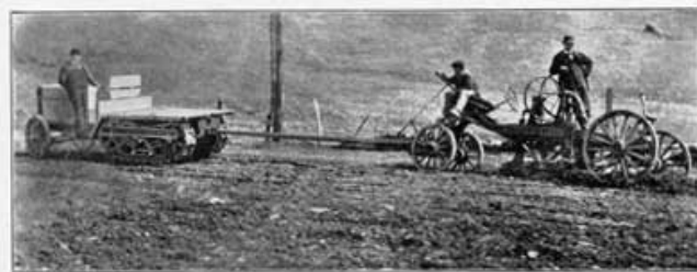
The Linn Tractor hauling with ease a heavy type of Road Machine on the highway with its blade down to a maximum depth. This photo was taken when the machines were at actual work on the road.
