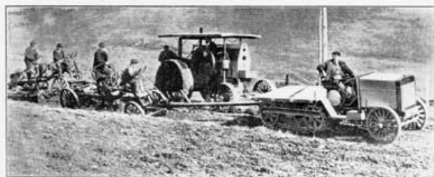
The Linn Tractor at work on the Highway doing far more efficient service than horses or a high wheel tractor. In fact the day this photo was taken the Linn Tractor hauled the high wheel tractor out of the ditch three times, where it had become helplessly stuck in soft ground. Plate Seven
