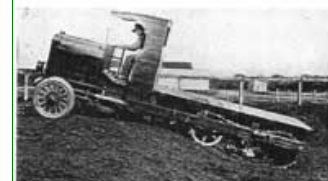
Illustrating the flexibility of the Linn traction member, maintaining full bearing on the ground.
