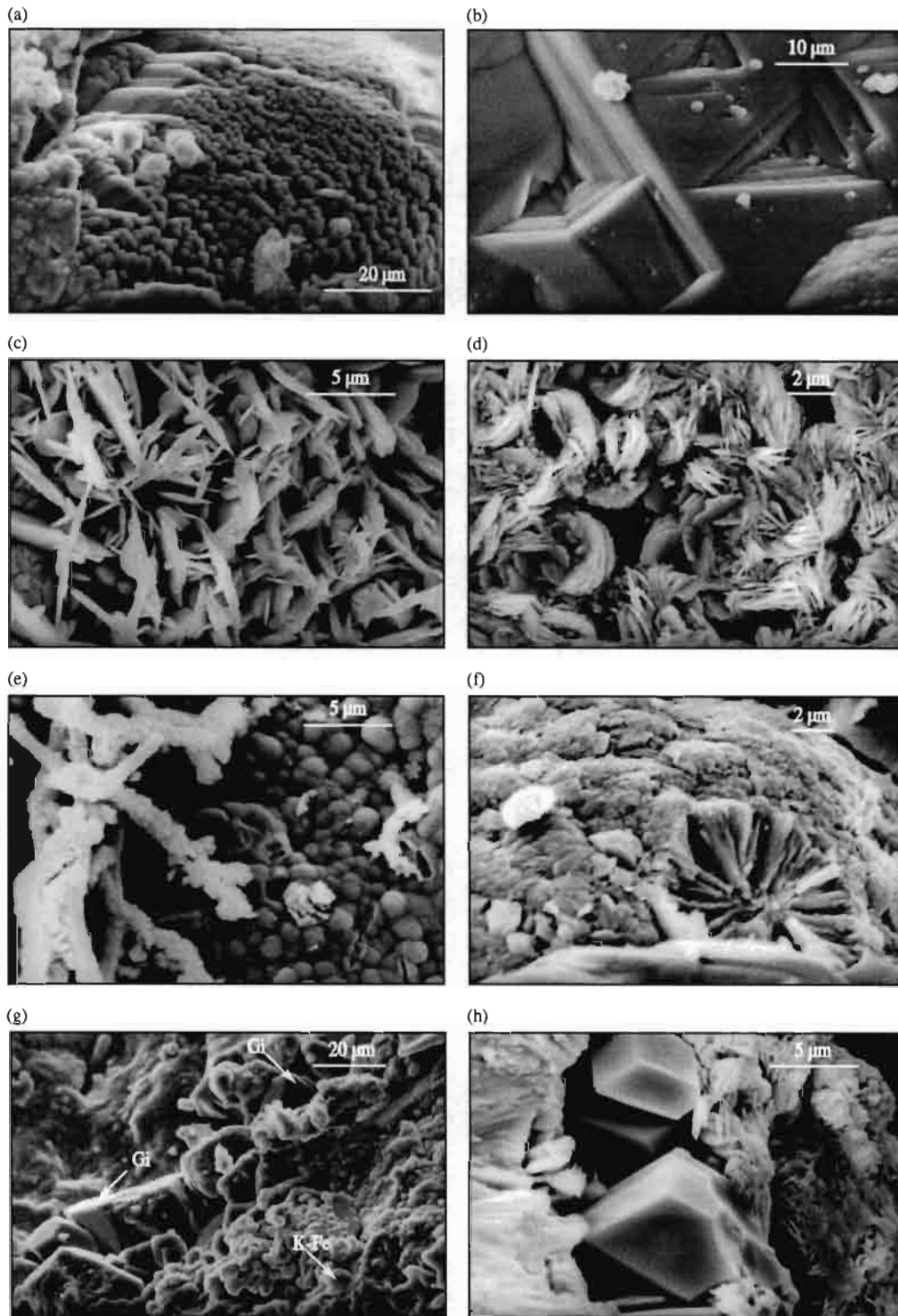
Figure 4 SEM images of quartz, haematite, goethite and gibbsite in ironstone gravels and iron pans: 'Floating' quartz in a gravel showing geometric forms (pyramids) in (a) relief and (b) depression. Coatings in iron pans made of thin (c) or thicker (d) platelets of haematite grouped in rosette. (e) Coating in iron pans made of acicular glomerules of goethite (background) and granular iron oxides on twisted stalks (foreground). (f) Detail of a glomerule with a broken zone showing radial distribution of needle-like goethite. (g) Void in iron pan with fine-grained iron oxides coating kaolinite (K-Fe) and growth of gibbsite crystals (Gi). (h) Detail of gibbsite crystals in a void with needle-like goethite (left-hand side of the void) and platelets of haematite (right-hand side of the void).
