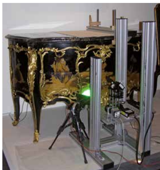
Fig. 2. Digital speckle pattern interferometry system used to diagnose damage areas in the lacquer layer of the commode – the investigated field is illuminated by a laser beam
