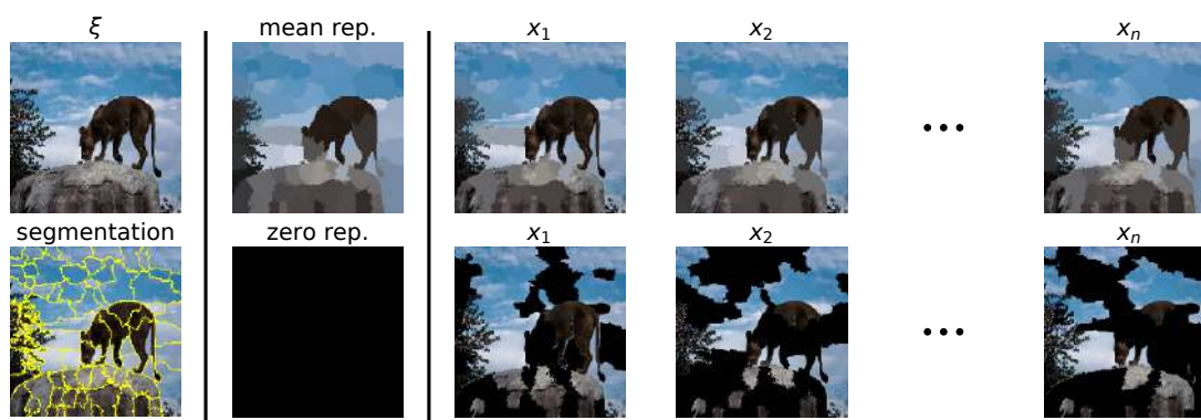
Figure 1: Sampling procedure of LIME for images. The image to explain, \xi , is first split into d = 72 superpixels ( lower left corner ). A replacement image \bar{\xi} is computed, which is by default the mean of \xi on each superpixel ( top row ). This replacement image can also be filled uniformly with a pre-determined color ( bottom row : replacement with the color black). Then, for each new example x_i with 1 \leq i \leq n , the superpixels are randomly switched depending on the throw of d independent Bernoulli 1/2 random variables.
