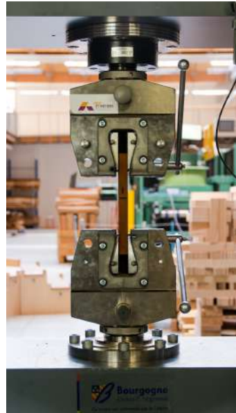
Universal Testing Machine "ZWICK" (compression, tensile and pressure tests)
