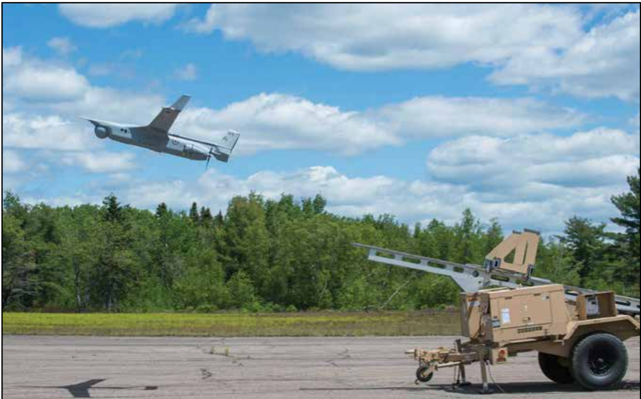
After being prepared by the maintenance crew, the new Blackjack SUAS is launched in the air for the very first flight of the Acceptance Test.
