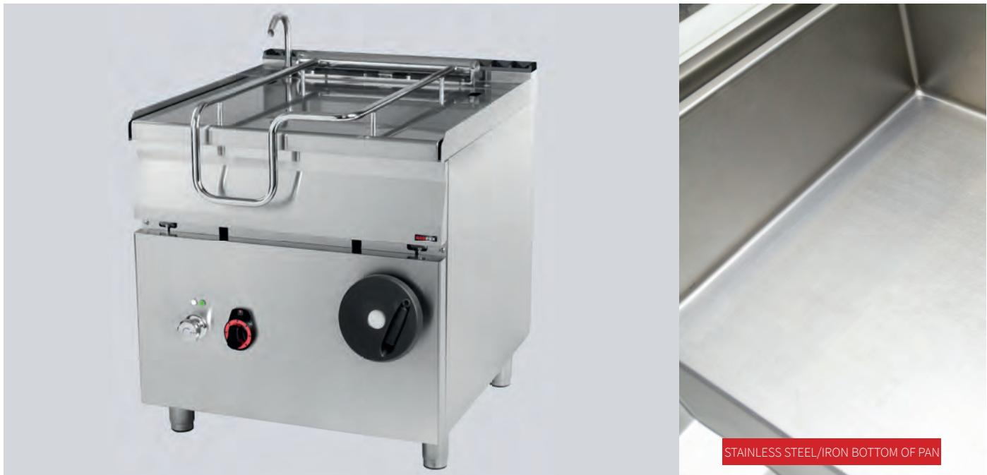
Tank, covering lid and front panel made of AISI 304. Optional steam collector inside a lid is available. Resistance or gas burner covers whole area of tank bottom, with no obstruction (the bracket of tilting system is fixed to the side part of tank). Two versions of tilting system – smooth manual operation or fully motorized tilt by a pushbutton switch.
