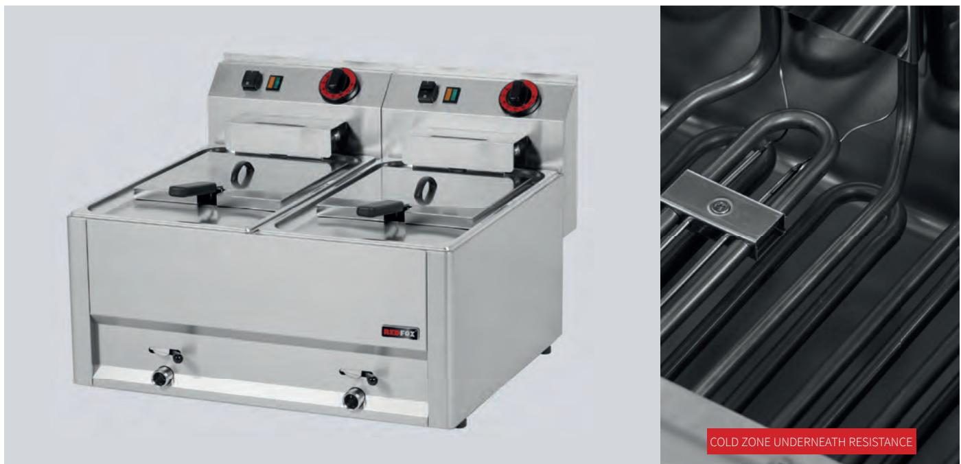
Pressed basins with ergonomic inner shapes and angles for comfortable cleaning and maintenance. Basin and top plate made of AISI 304. The choice of different power outputs, basin volumes and basket configurations enables you to select the best combination for your operation. Solid support of heating elements ensures a proper cold zone underneath resistances. Safety thermostat for safe operation. Solid construction of baskets and long resistances (large surface) for long lifetime of components.
