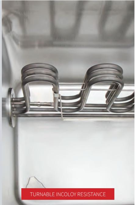
Pressed basins with ergonomic inner shapes and angles for easy cleaning and maintenance. Basin is made of AISI 316 and front panel made of AISI 304, thickness 1,5 mm. Equipped with water filling system, smooth thermoregulation 30 – 110 °C and safety thermostat 130 °C. Rotating heating element is made of Incoloy 820. Different shapes and sizes of baskets provide many variations and configurations suitable for any catering unit.
