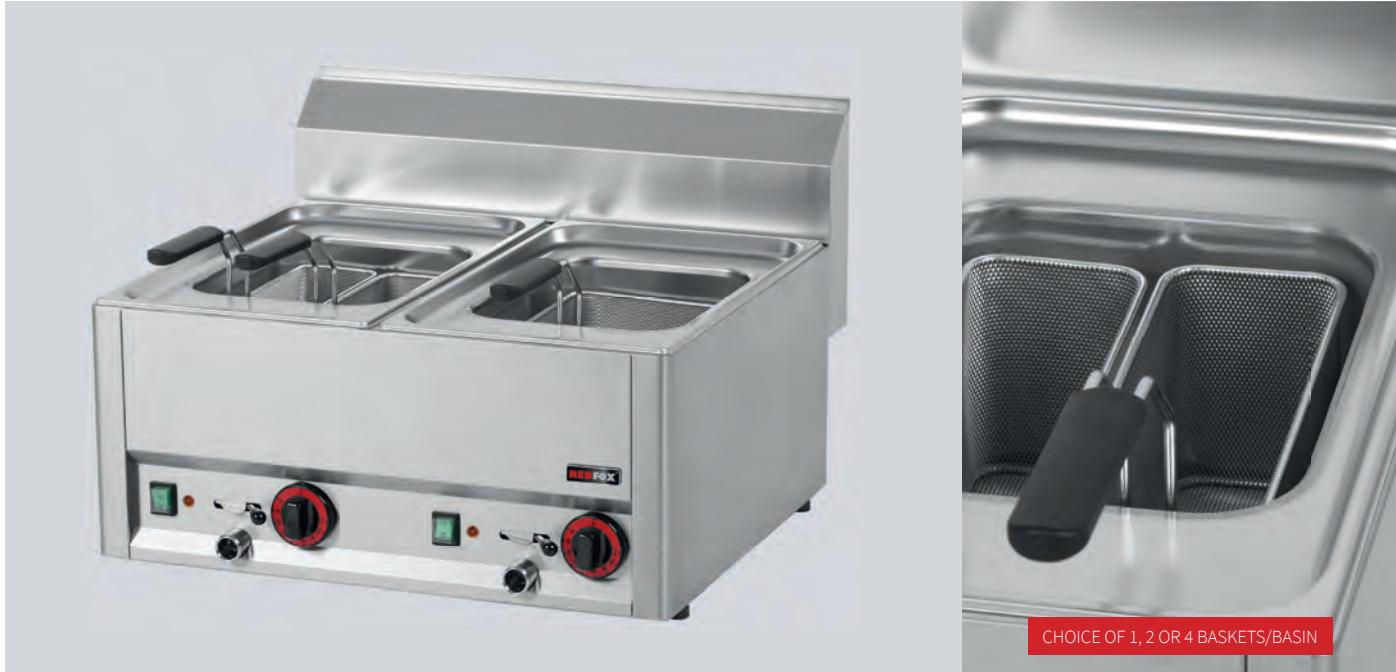
Pressed basins with ergonomic inner shapes and angles for easy cleaning and maintenance. Basin and front panel made of AISI 304. Smooth thermoregulation 30 – 110 °C and safety thermostat 130 °C. Heating element is made of Incoloy 820. Three different shapes and sizes of baskets provide many variations and combinations.
