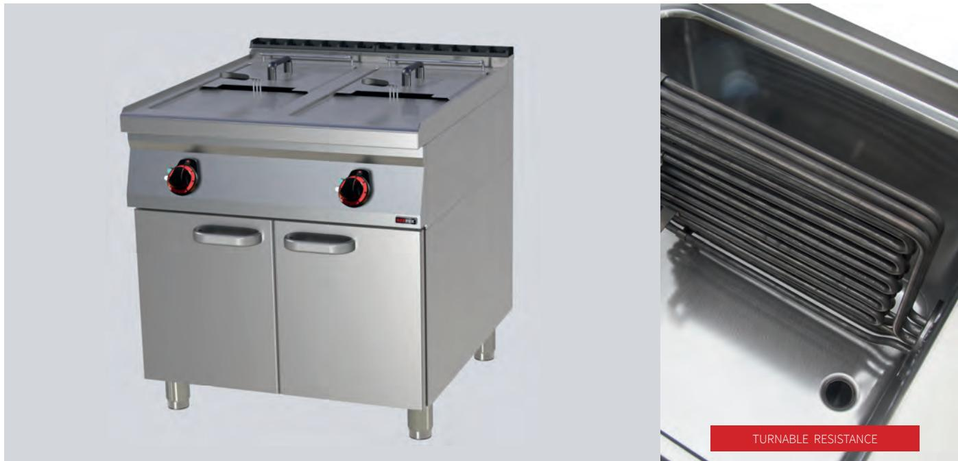
Pressed basins with ergonomic inner shapes and angles for easy cleaning and maintenance. Basin and front panel made of AISI 304, thickness 1,5 mm. Rotating resistances with a solid support, ensuring a proper cold zone underneath. Oil drainage into the GN basin inside neutral cabinet.
