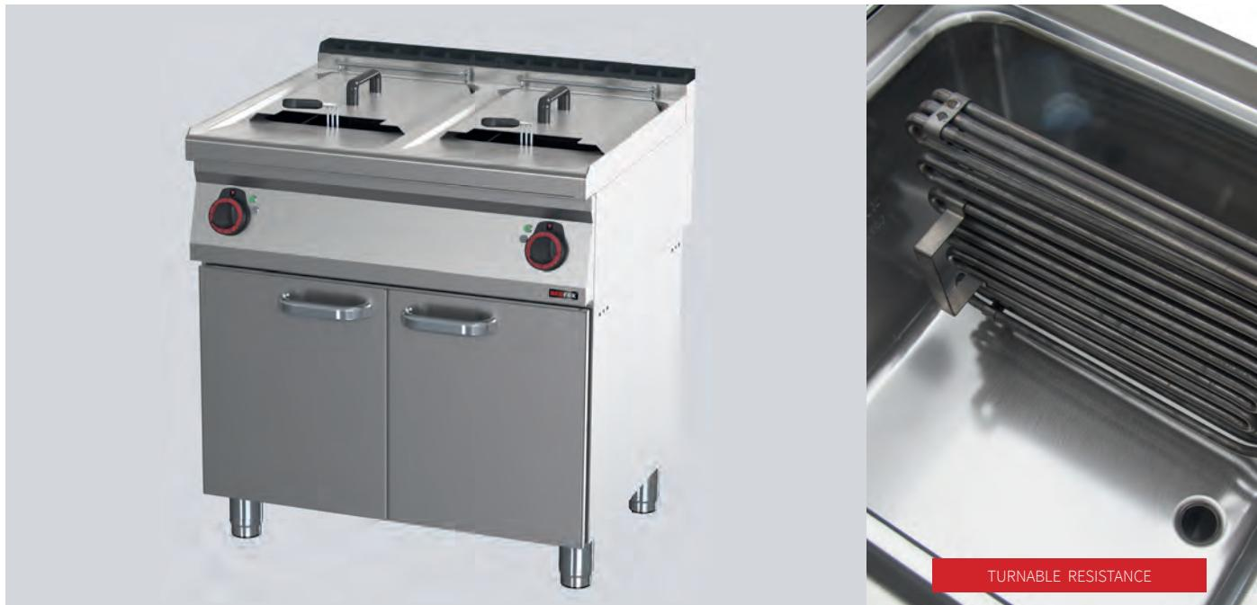
Pressed basins with ergonomic inner shapes and angles for easy cleaning and maintenance. Top plates are made of AISI 304. Top plate thickness is 1,2 mm. Selection of different power outputs and basin volumes. Rotating resistances with a solid support, ensuring a proper cold zone underneath. Oil drainage into the GN basin inside neutral cabinet. Standard sizes of 400 and 800 mm in width.
