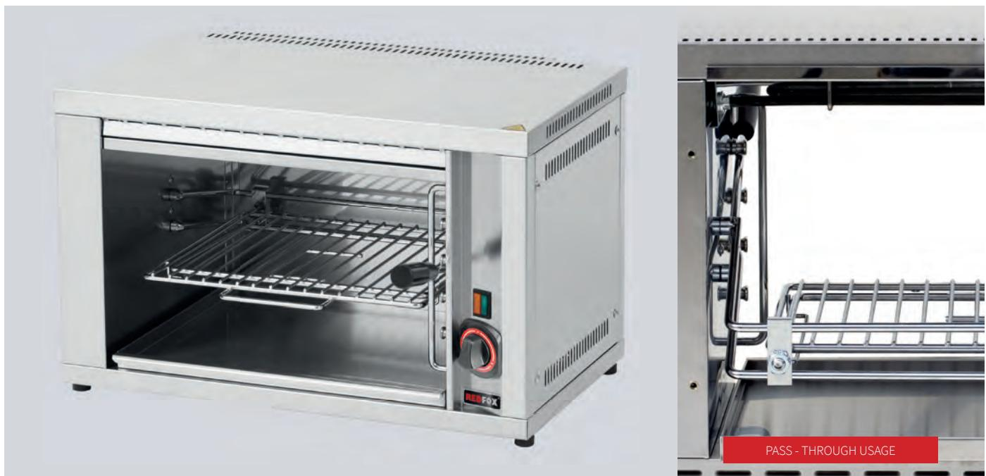
High-temperature proof resistances are made of material Incoloy 800. Heat performance is regulated by the energy regulator. 2 options of grid mechanism – basic manual pull-out positioning or smooth adjustment by a lever and pre-set 4 height-positions. Appliance is suitable for finishing meals, gratinating, browning and keeping meals at serving temperature. Back side panel may be removed away so the device becomes a pass-through option between the chef's kitchen and the serving area.
