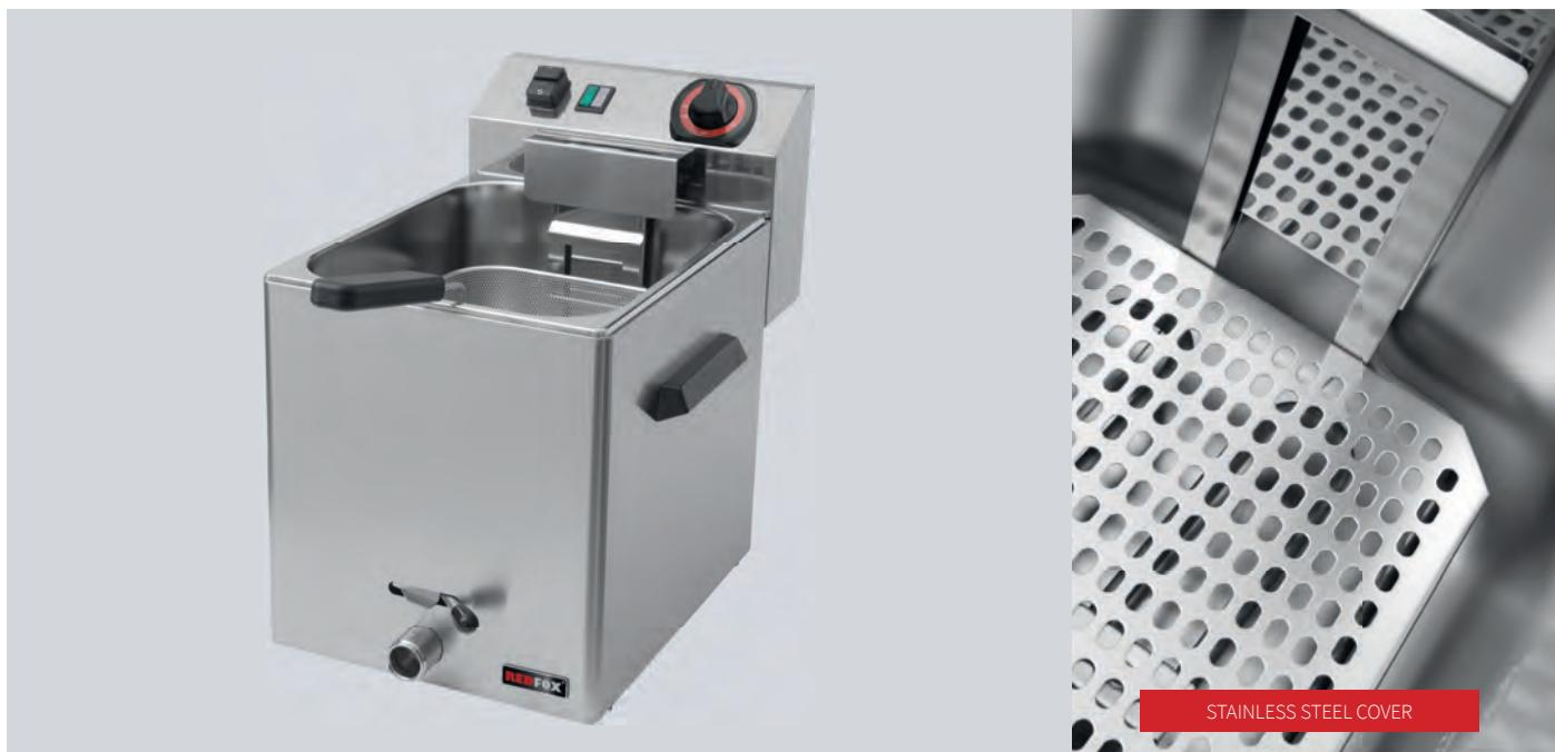
Heating element made of Incoloy 820, resistant to high salt concentration. Pressed basin with ergonomic inner shapes and angles for comfortable cleaning and maintenance. Basin is made of AISI 304. Drain tap with safety arm device. Stainless steel panels covering the resistance against damage or bending. Security thermostat set up for 130 °C.
