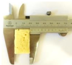
Figure III-21: Picture of measuring of volume of PHU foam
