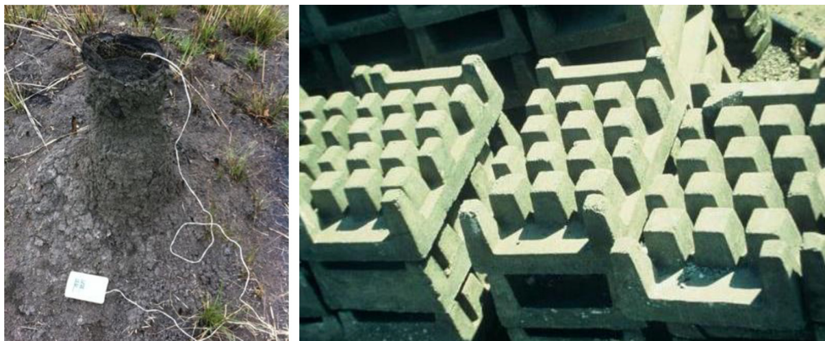
Fig. 4. Temperature measurements of termite mounds carried out by Mick Pearce (left), CC-SA-BY Licence, Mick Pearce. (b) Heat exchange floor under construction, abstraction of the biological principles of termite mounds, CC-SA-BY Licence, Mick Pearce.
