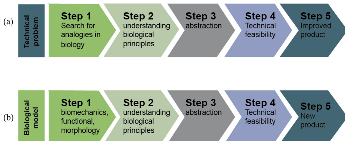
Fig. 1. Biomimetic design process. (a) technology pull, (b) biology push. Adapted with permission from ISO standard 2015:18458 [2].
