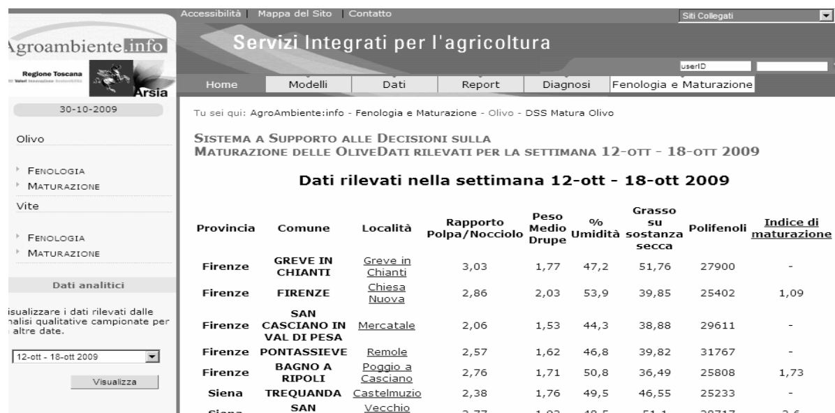
Figure 5: the page reporting the physical-chemical data for olive fruit ripening on each site monitored. In this example the data for the week 12-18 October are shown.
