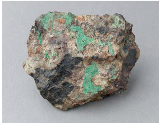
FIG. 2.1. Uraninite (pitchblende) with torbernite from the collection of Martin Klaproth (reproduced with permission courtesy of Museum für Naturkunde, Berlin, Inv. No. MFN_MIN_1985_006, photo: © Hwa Ja Götz, MfN).
