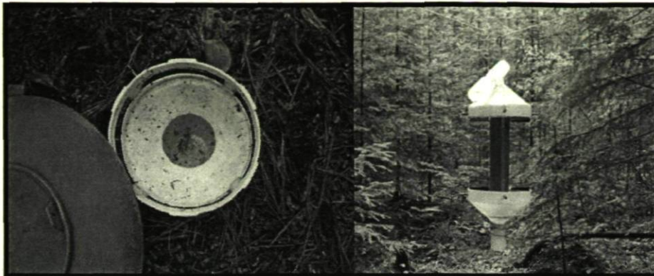
Figure 2-3: Left, the pitfall trap. Right, the multidirectional flight-interception trap.
