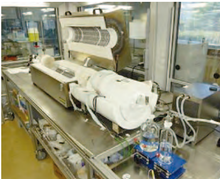
Figure 1 START: Study of the Transport of RuThenium on the primary circuit, an OCDE/STEM project is an experimental study in order to measure quantification and deposition of ruthenium under primary circuit conditions.
