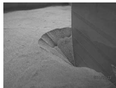
Figure 5. A close-up photo of the upstream inverse conical shape at H=36.78 cm (E0317)
