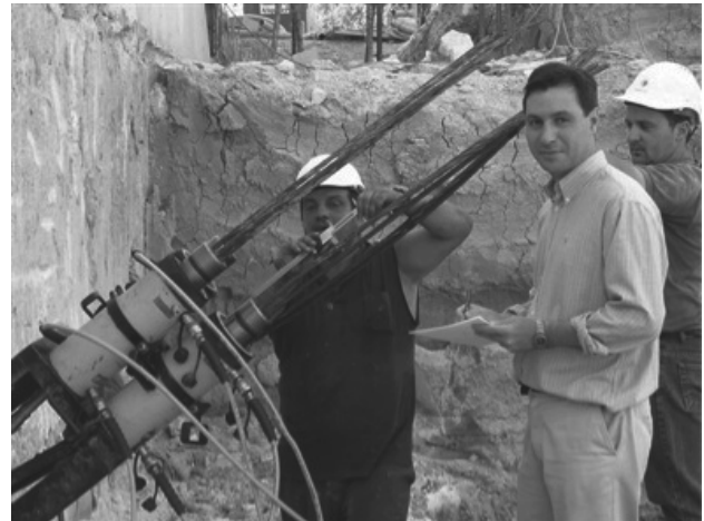
Figure 5. Trial research test with multiple synchronized hydraulic jacks in Parking La Vega, Murcia, 2005.
