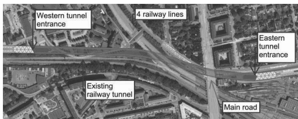
Figure 1. Horizontal alignment and key structures.
