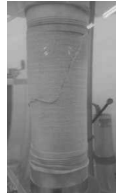
Photo 2. Condition of the test specimen after shear
