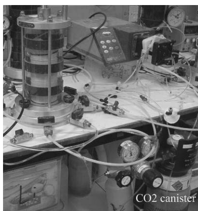
Figure 1. The triaxial cell used for MgO-stabilised soil carbonation.
