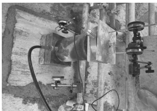
Figure 2. Typical set-up for pull-out tests.
