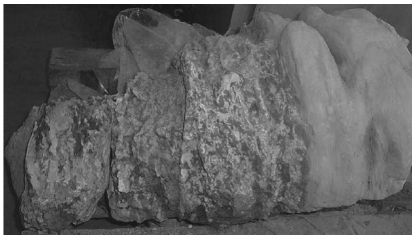
Figure 5. Structure of excavated jet grouting column (photo: J. Bzówka).
