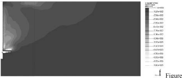
7. Radial stress contour plot at the onset of failure.
