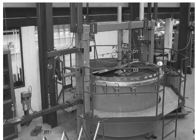
Figure 2. Test setup for cyclically long-term loaded monopiles.
