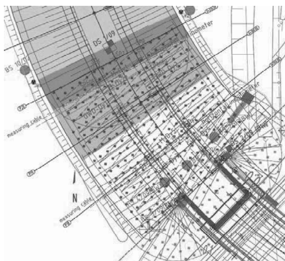
Figure 1. detail of the highest embankment west with the bridge abutment over the highway B5 (CMC close to bridge and coloured areas with vertical drains and preloading)
