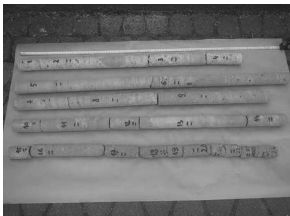
Figure 1. Core samples for strength tests (Bzówka, 2009).
