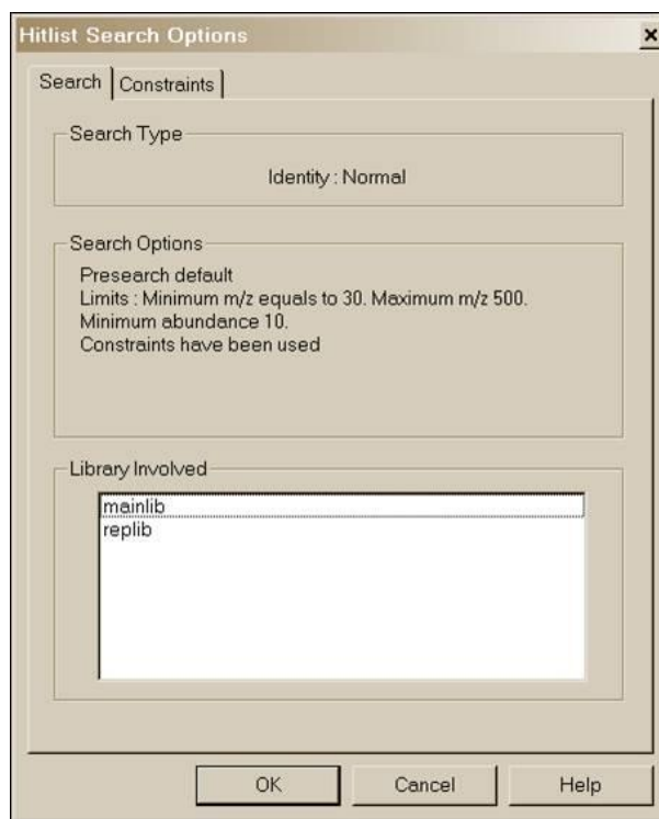
Figure 11. List of libraries used in a Library spectrum Search along with the Search Options
