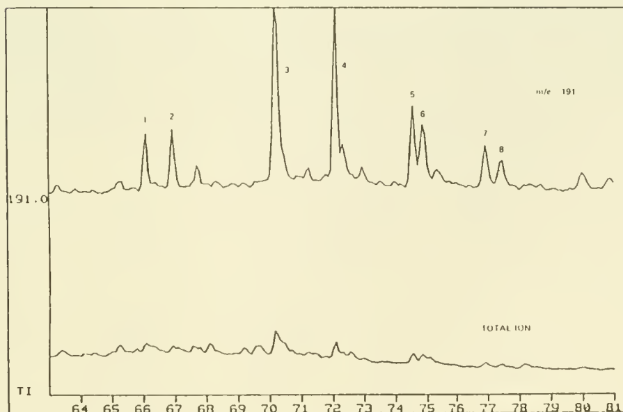
FIGURE 3.4. Triterpane ( m/e 191) mass chromatogram of weathered oil. 1,2 = Trisnorhopane ( C_{27}H_{46} ), 3 = Norhopane ( C_{29}H_{50} ), 4 = Hopane ( C_{30}H_{52} ), 5,6 = Homohopanes ( C_{31}H_{54} ), 7,8 = Bishomohopanes ( C_{23}H_{56} ).
