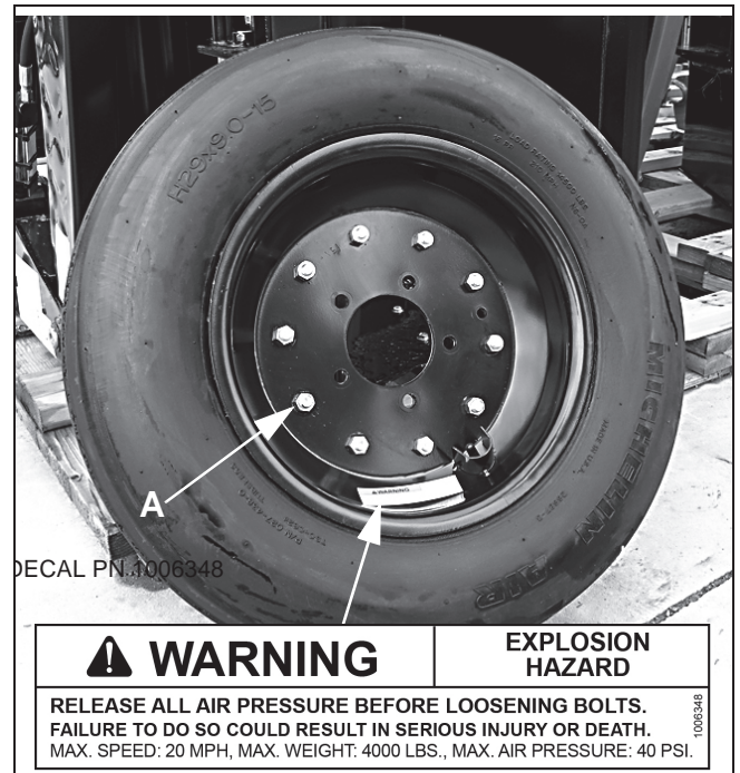
Figure 16. Split Rim Tire Servicing
