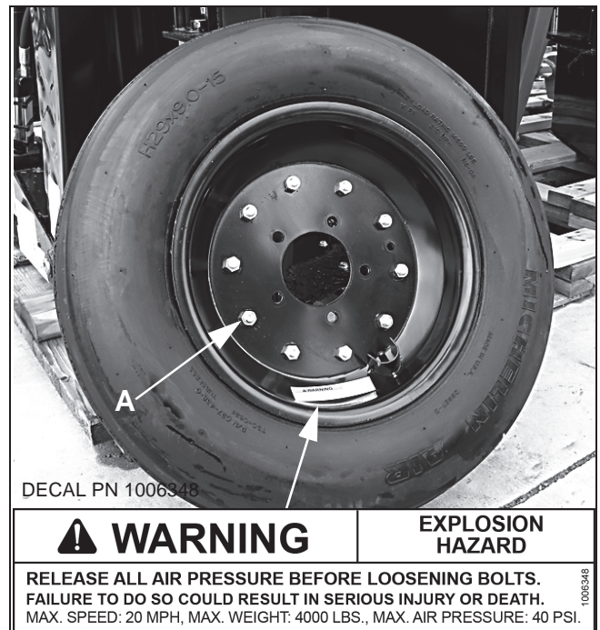
Figure 33. Split Rim Tire Servicing
