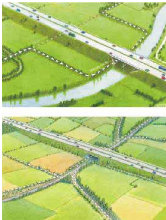
Figure 5 : Tunnels for water courses or smaller secondary roads can be designed to provide a safe underpass for bats
