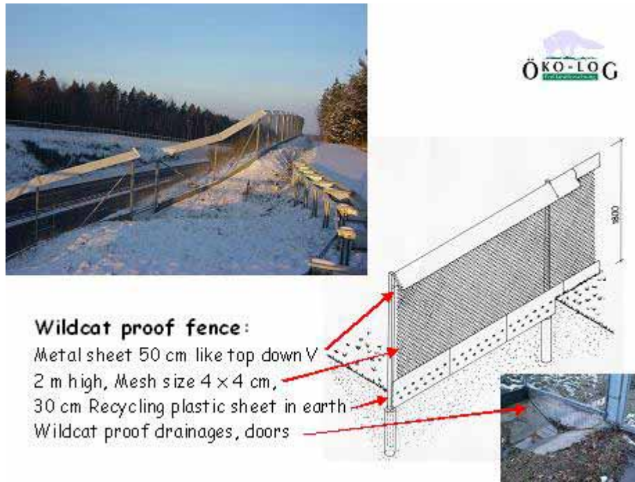
Figure 3 : The wildcat proof fence and its construction
