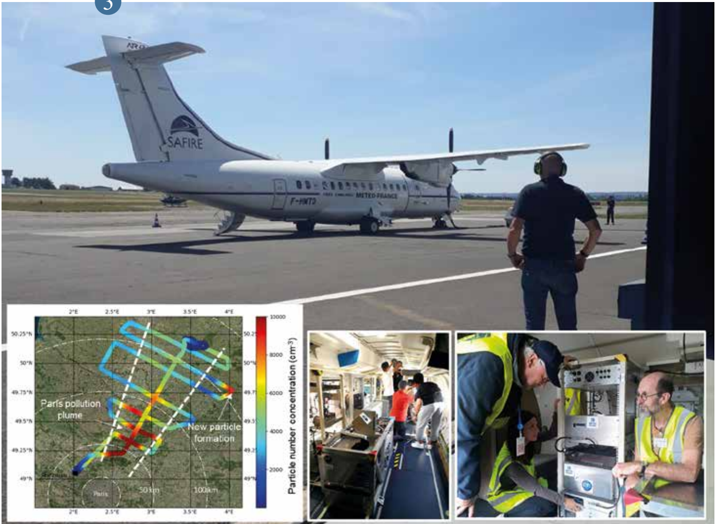
Main figure: Preparation of the SAFIRE ATR-42 research aircraft before take-off. Bottom left: Particle number concentration measured during a scientific flight. Bottom middle figure: Preparation of the instrumentation on board the aircraft. Bottom right: Calibration of the HTDMA-SP2 newly developed by CNRM.
