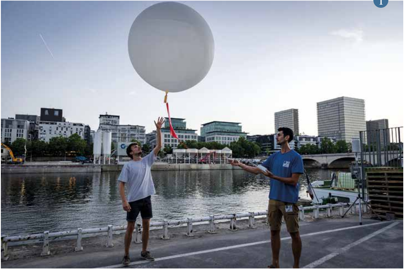
▲ Launching of a weather balloon to observe the vertical structure of the urban heat island from the Bercy quays (photo credit: Cyril Fréssillon, CNRS).
