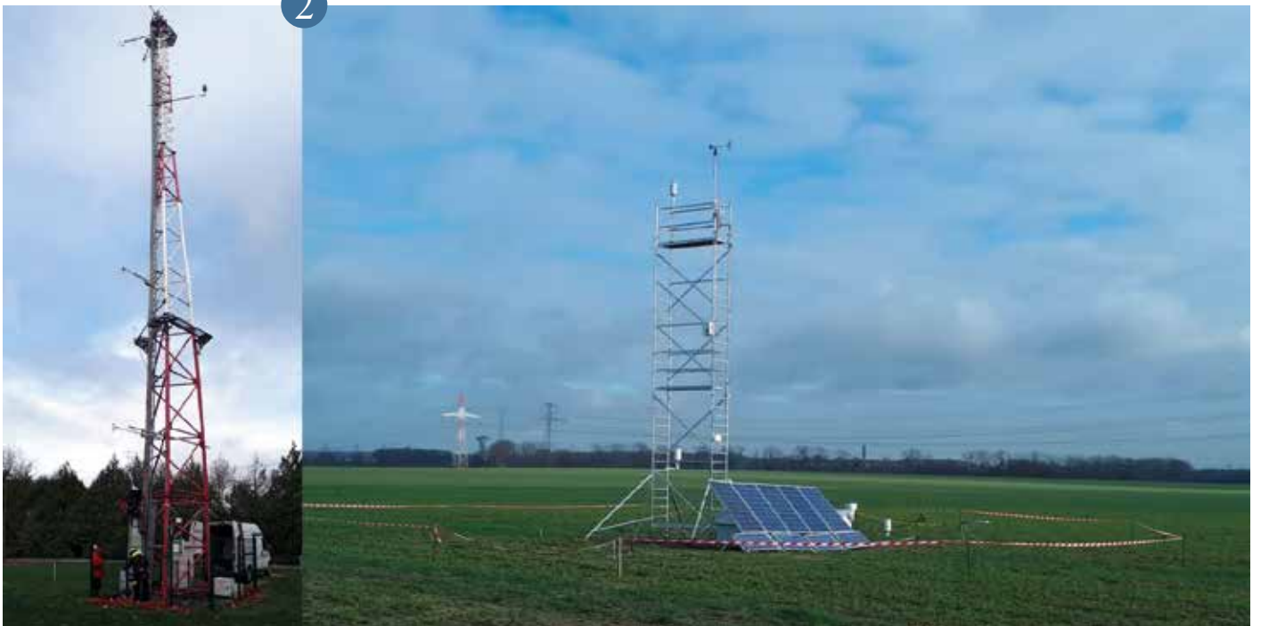
▲ Surface Energy Budget station (left) on a 30m mast on the Polytechnique site, (right) in the middle of an agricultural field on the Saclay plateau.
