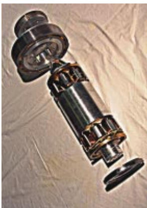
The passive parts of the radial magnetic bearings on both ends of the axis, and the axial bearing.
