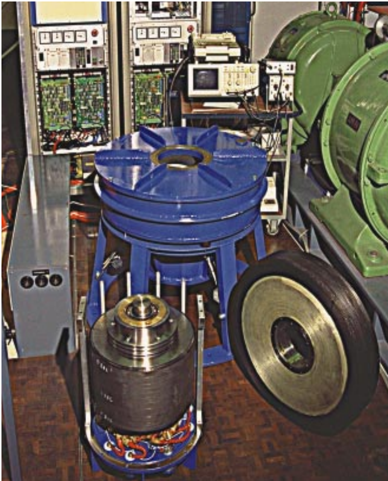
The system's components: in the left background the racks with power electronics and controls, in the centre the casing with base, in the right foreground the motor/generator, at right the flywheel (bright coloured inner part: glass fibres, dark coloured outer part: carbon fibres)
