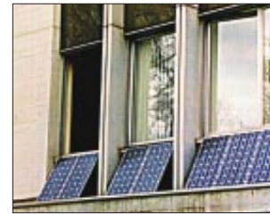
Above: Crystalline laboratory modules exposed to durability tests in the open air.
