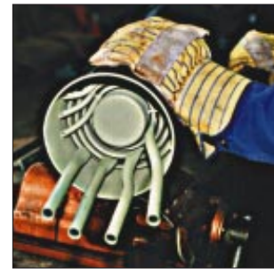
Top: Looking down into the absorber, where the »poor« solution again enriches itself with ammonia.
