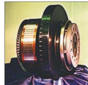
The flywheel (left), and attached to it the rotor of the electric machine (left), and the clutch (right) between the flywheel and the CVT.
