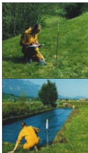
Top: For gas sniffing, probes are inserted into the soil.
