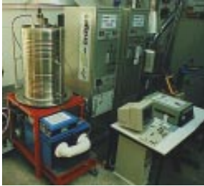
Above: HEXIS test laboratory in Winterthur. On the left the thermally insulated cylindrical casing of the 43 cell stack. On the right, electronic controls and measurement equipment.
