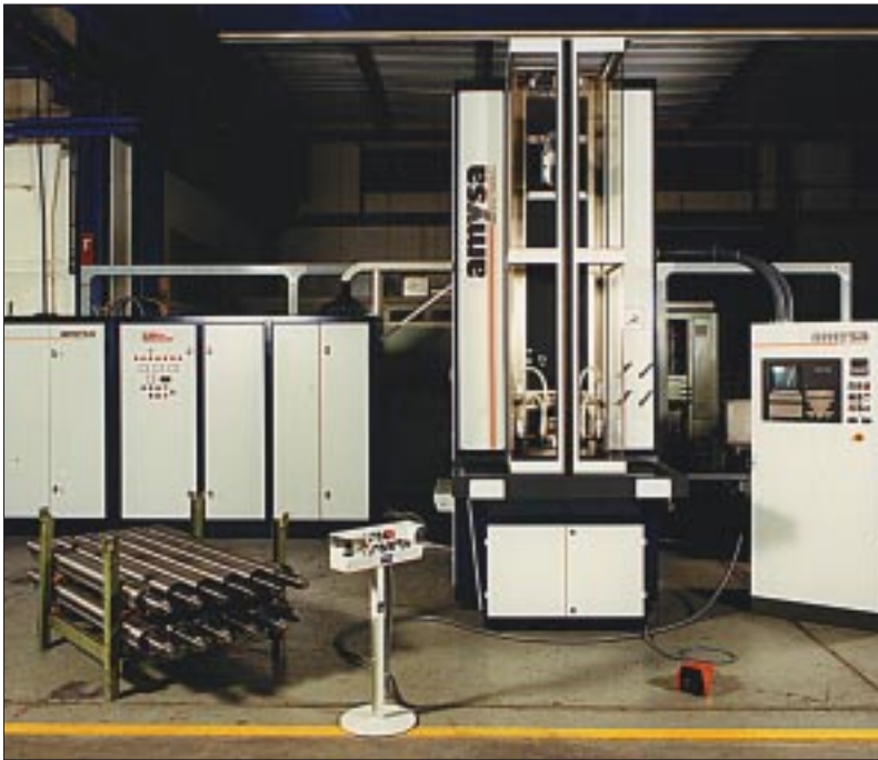
Industrial induction heating machine designed according to the findings of the NEFF project. Right of the centre is the induction furnace proper, in which the induction coils move vertically. At the right, and in the left background, is the electronic control of the machine. In the foreground at left are workpieces prepared for induction treatment.
