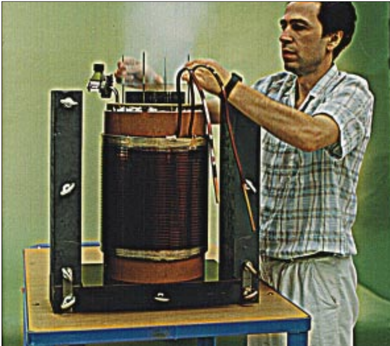
The 100 kVA device after assembly. On top is the cryostat with attached connecting tube (left) for pumping down the vacuum chamber. The iron yoke has yet to be added.
