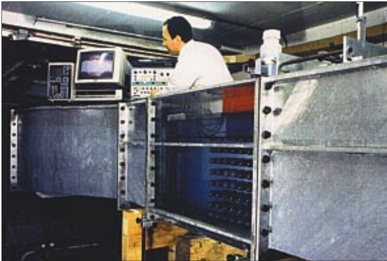
In the water channel facility, side walls and top cover made of perspex enable the observation of unsteady flow structures. In the middle there is a tube array (here in-line) of horizontally mounted rods. Placed on top of the channel are components of the video system.
