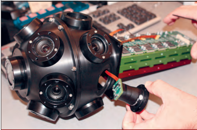
Figure 2. R7 Street View camera system. The system is a rosette (R) of 15 small, outward-looking cameras using 5-megapixel CMOS image sensors and custom, low-flare, controlled-distortion lenses.
