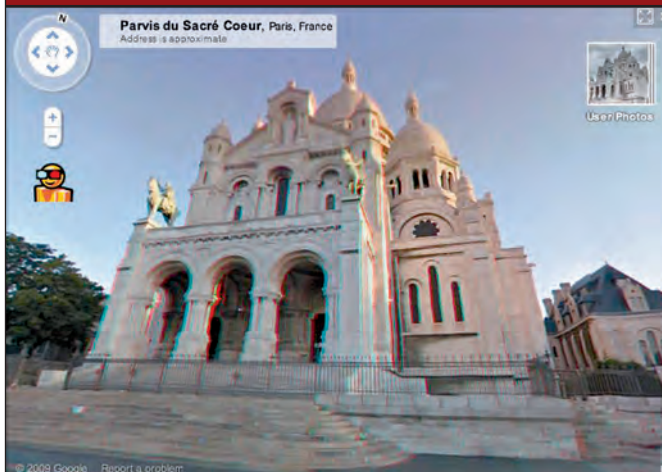
Figure 7. Panoramic 3D anaglyphs let users experience depth in Street View with simple red-cyan eyeglasses. Known depth is used to synthesize binocular parallax on the client side, thereby creating a second displaced view that replaces the red color channel in the original view.
