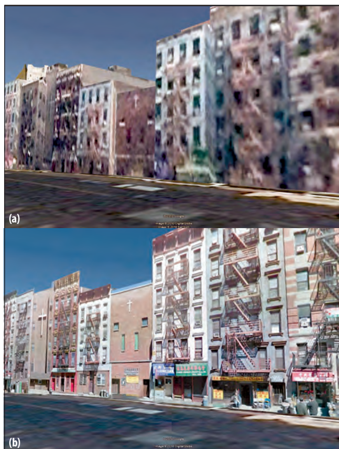
Figure 8. Using Street View data to enhance user walk-through experiences in Google Earth. (a) Original 3D models of a New York City scene from airborne data only. (b) Fused 3D model with high-resolution facades. The visual quality is considerably higher, and many storefronts and signs can be easily identified and recognized.
